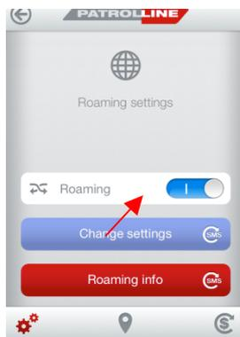
By pressing "Roaming" menu, you will see setting roaming possibilities, allowing or denying the roaming traffic cost of the SIM card.
