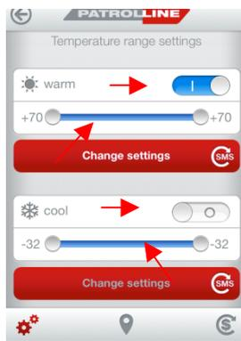
pressing "Temperature Range" menu, you will see setting possibilities (Summer/Winter) and here you can fix the desired temperature range during the remote control engine start function.
