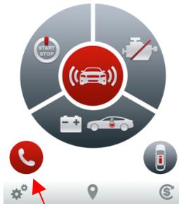
pressing "e" icon you can the alarm system and, after 4 rings, you can listen what's happening inside the car (silent mode). If you close the call at the second ring, the system will tell you: 1) status of the system; 2) status of the engine; 3) battery voltage; 4) dashboard temperature.
